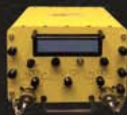
AN/ALM-295 Countermeasures Dispenser Test Set (CDT)
